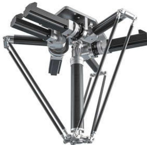
*Figure 1. 3. Robot parallèle, Robot Delta, (Paccot, 2009)*
