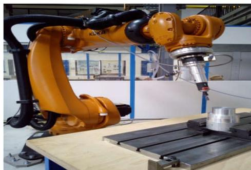
Fig. 4. Machining robot cell
