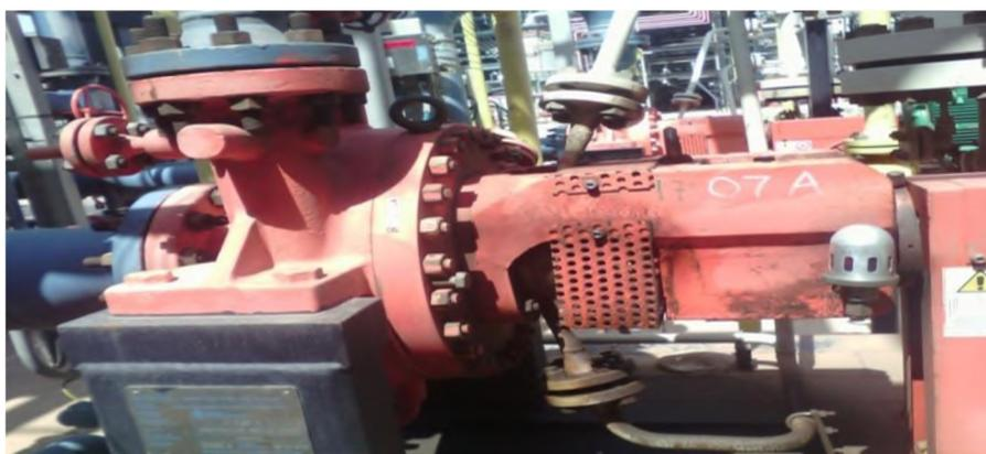
Fig 3. 10. Pompe centrifuge 17-MJ-07- A
