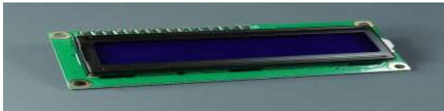
Figure 4-7: Afficheur LCD
