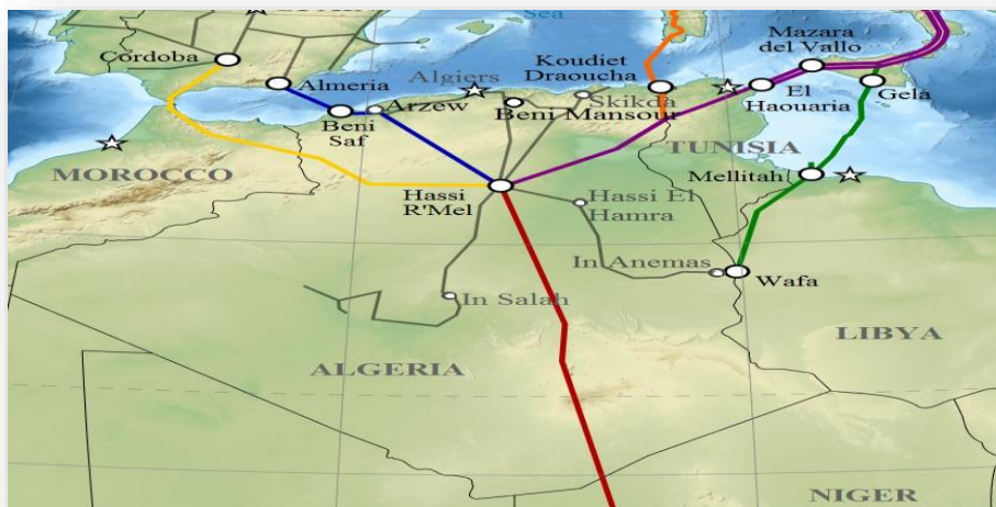
Figure 1.2 Trans-Mediterranean and future Trans-Saharan gas pipelines [8].
