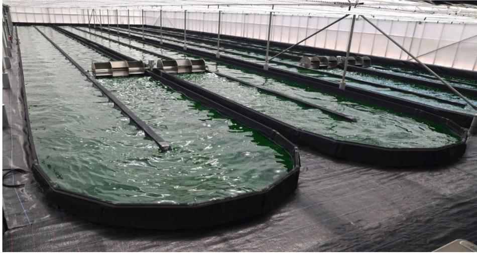
Figure II.19 : Bassin "raceway".[26]
