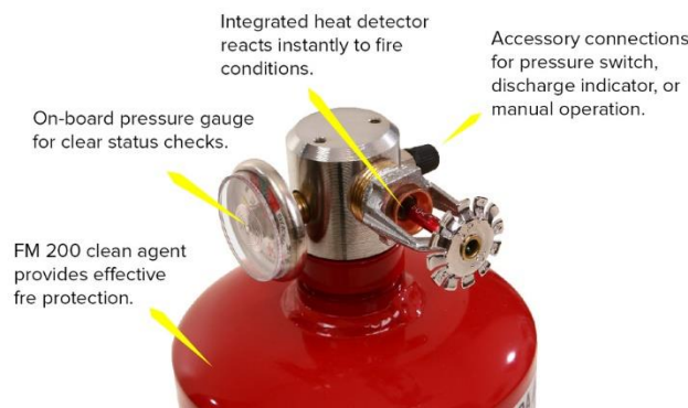
Figure III. 13: Automatic Fire Extinguishers for Fire Protection.
