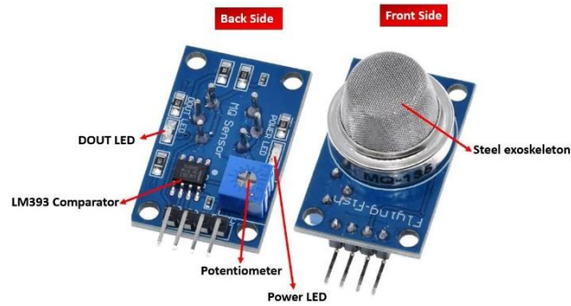
Figure III. 3: Interfacing of MQ-135 Gas Sensor with Arduino.
