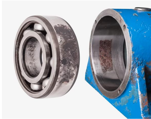
Figure II.9. Effet fretting corrosion [22]
