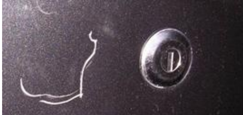
Figure II.15. Effet de rayage [22].
