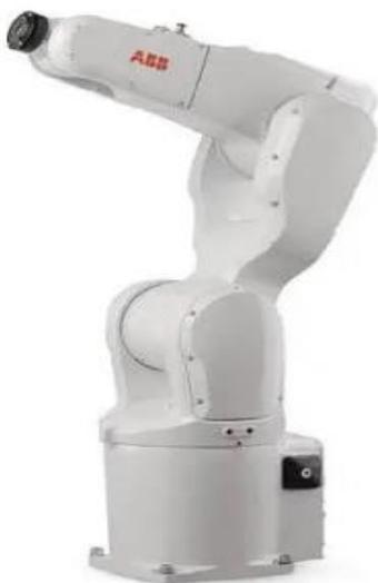
**Figure 4.2 :** Robot IRB 1200
