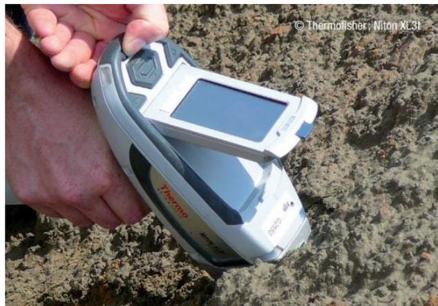
Figure 4 8:PXRF (field portable X-ray fluorescence)
