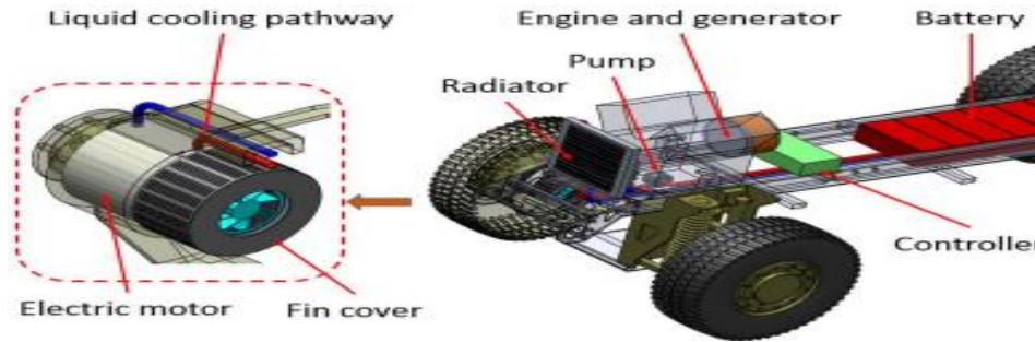
Figure 3-24 electric vehicle chassis schematic with liquid and heat pipe motor cooling.
