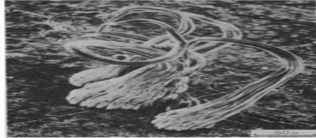
Figure 2-4 : Scanning electron micrograph of silver fibers resulting from reduction of silver sulphide with hydrogen at 500°C [52].
