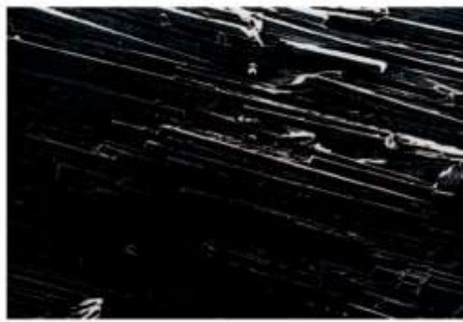
Figure II-1- Rupture fibre en traction[22]
