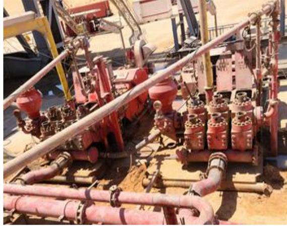
**Figure 6: pompes de forage [18]**
