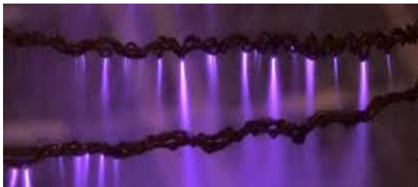
Figure 1-2: Electrode couronne à pointe
