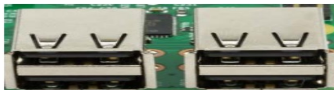
Figure III. 4: The raspberry pi USB interfaces.
