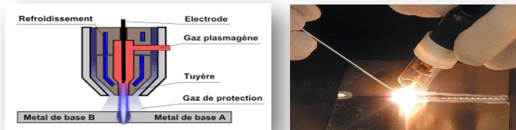
Figure I.10: Soudage plasma (PAW: Plasma Arc Welding)
