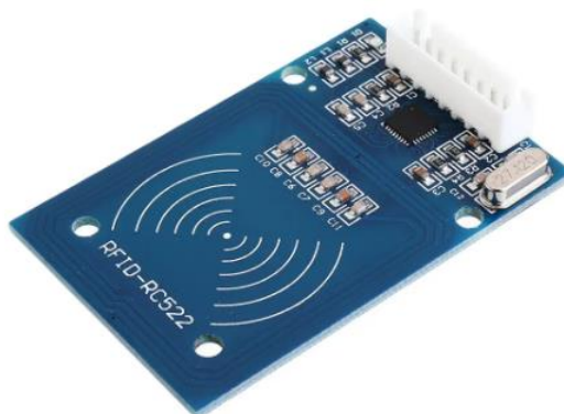
Figure III. 2: RC522 RFID Module.
