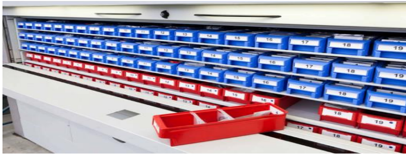
Figure I-7 Stockeur rotatif vertical GIROPHARMA
