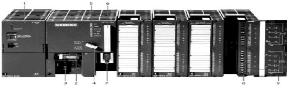
Figure 1.9: automate programmable industrielle SIEMENS
