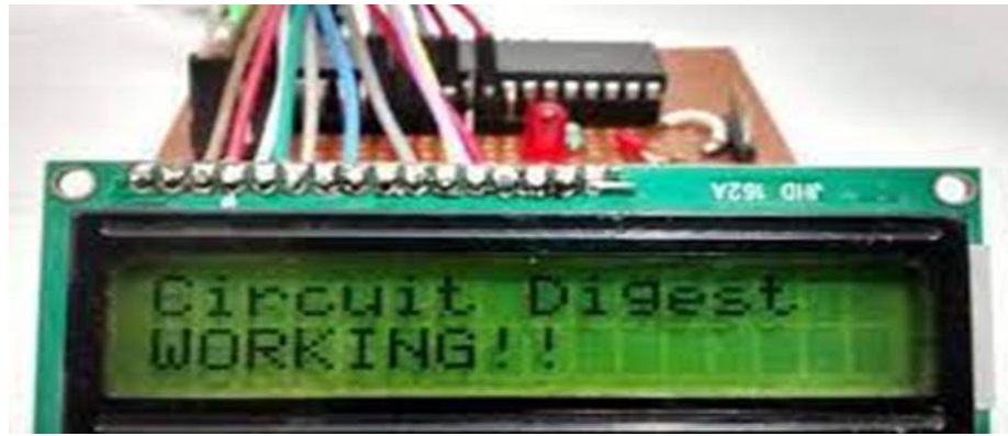
Figure II.5: LCD Display Interfacing With Pic Microcontroller
