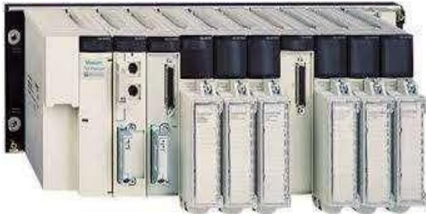
**Figure 1.18 :** Automate modulaire (Modicon).
