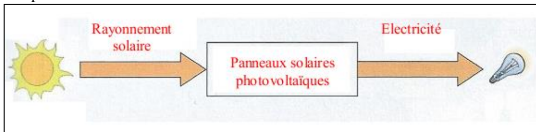
Figure II.21 : Energie solaire photovoltaïque
