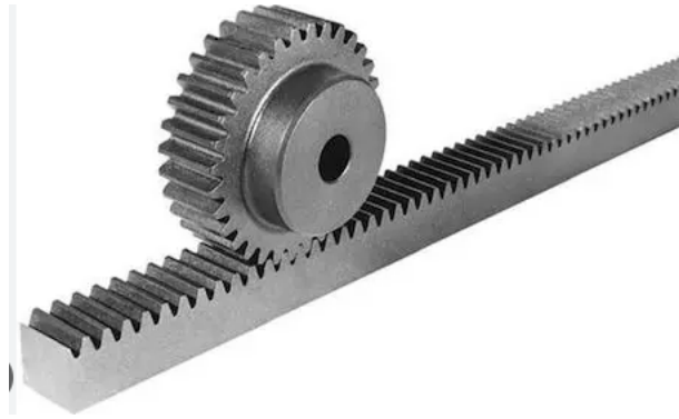
Figure 1.4: Rack and Pinion.[11]
