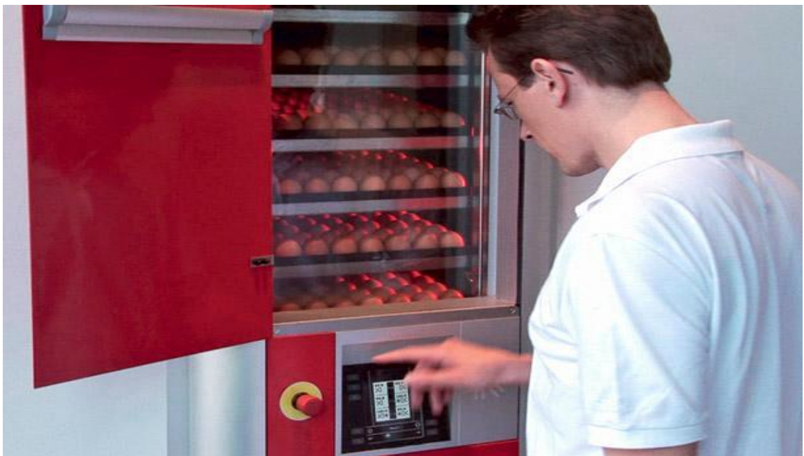
Figure I.21: Preheating the eggs before the incubation step
