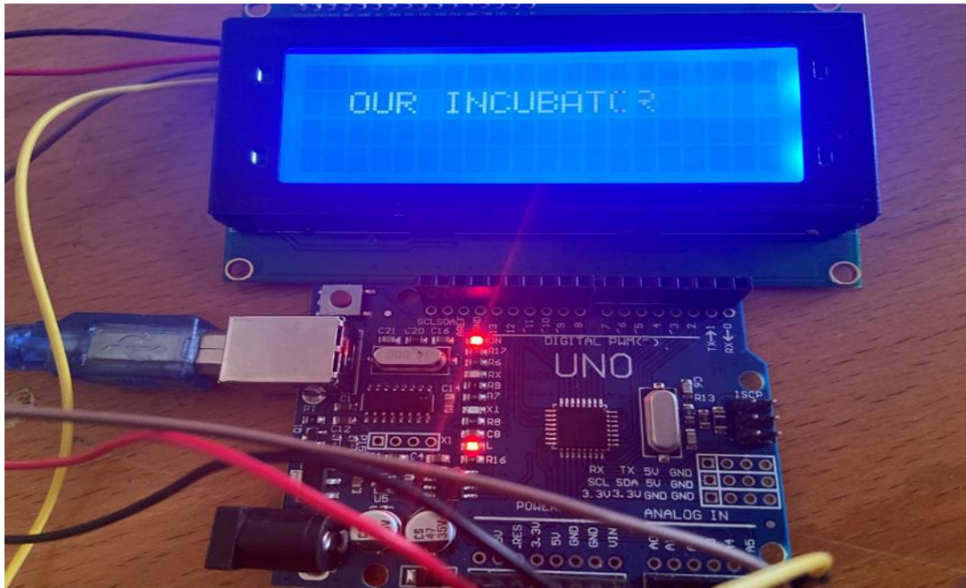
Figure IV.7: Connecting LCD to Arduino
