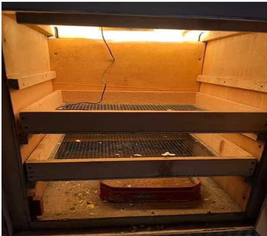
Figure I.9: The manual incubator
