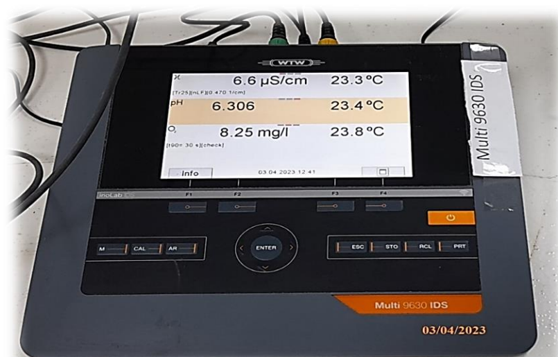
Figure 22 : Appareil Multi 9630 IDS (T°, pH)
