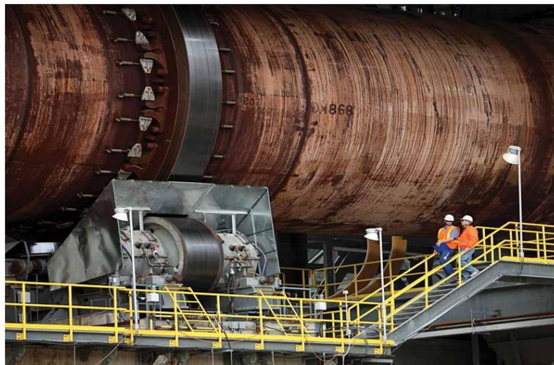
**Figure I.5 :** Station des galets.
