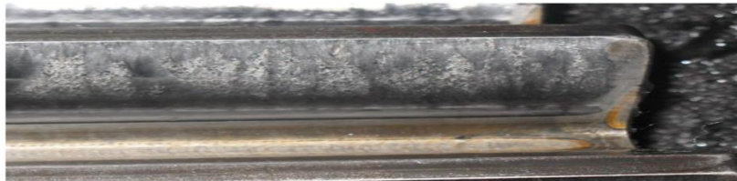
Figure III. 15. Le grippage "Engrenage" [15].
