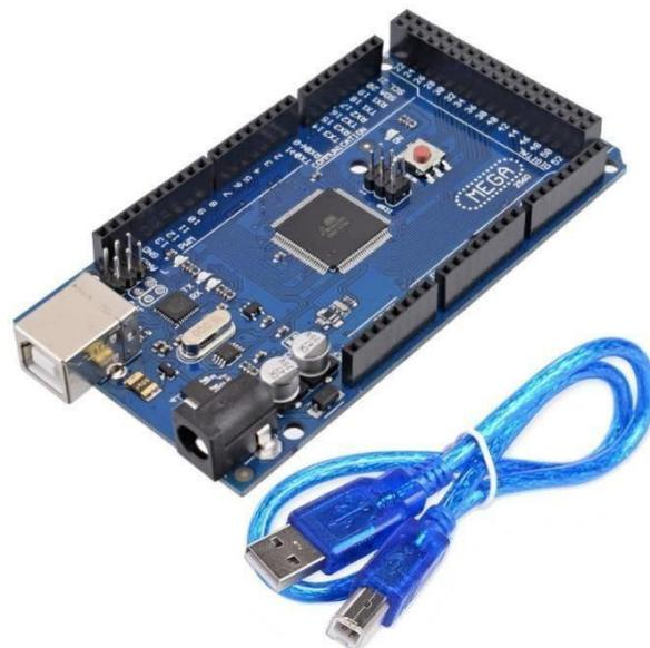
Figure III.5 : Arduino MEGA
