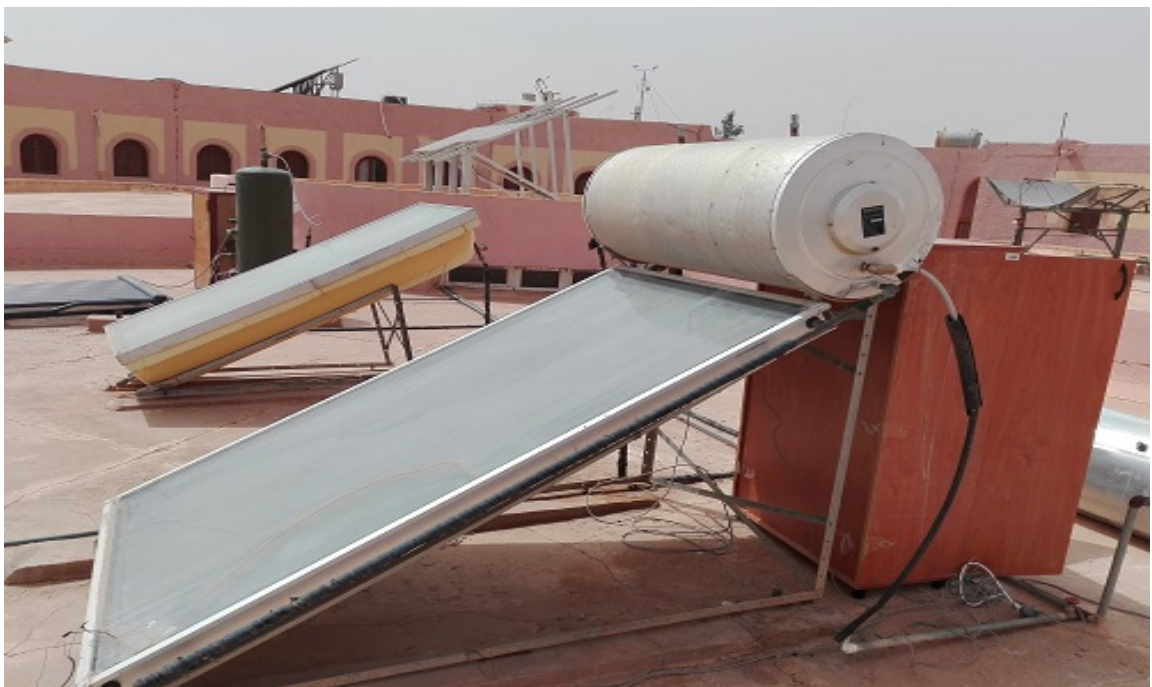
Figure 4.2 Photograph of the experimented flat plate thermal solar collector.
