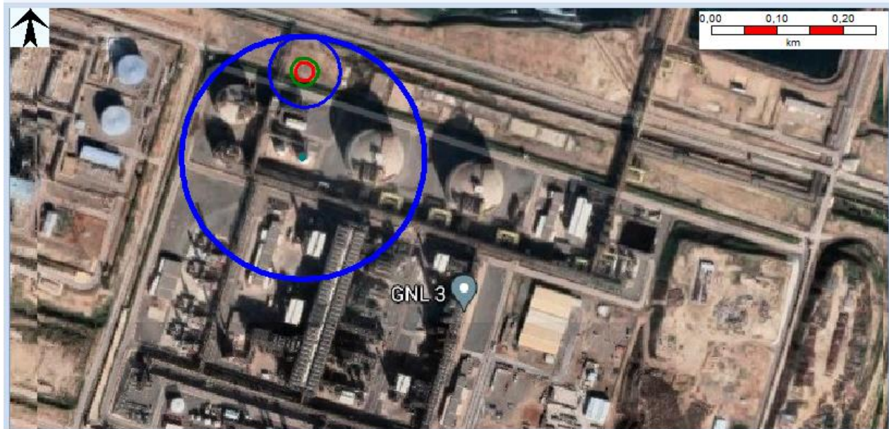
Figure 3- 19 Areas affected by thermal explosion effects in the 30mm-leak
