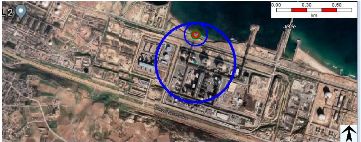
Figure 3- 29 Areas affected by thermal explosion effects in the 60mm-leak
