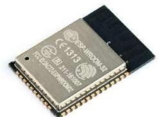
Figure 8. Module ESP32
