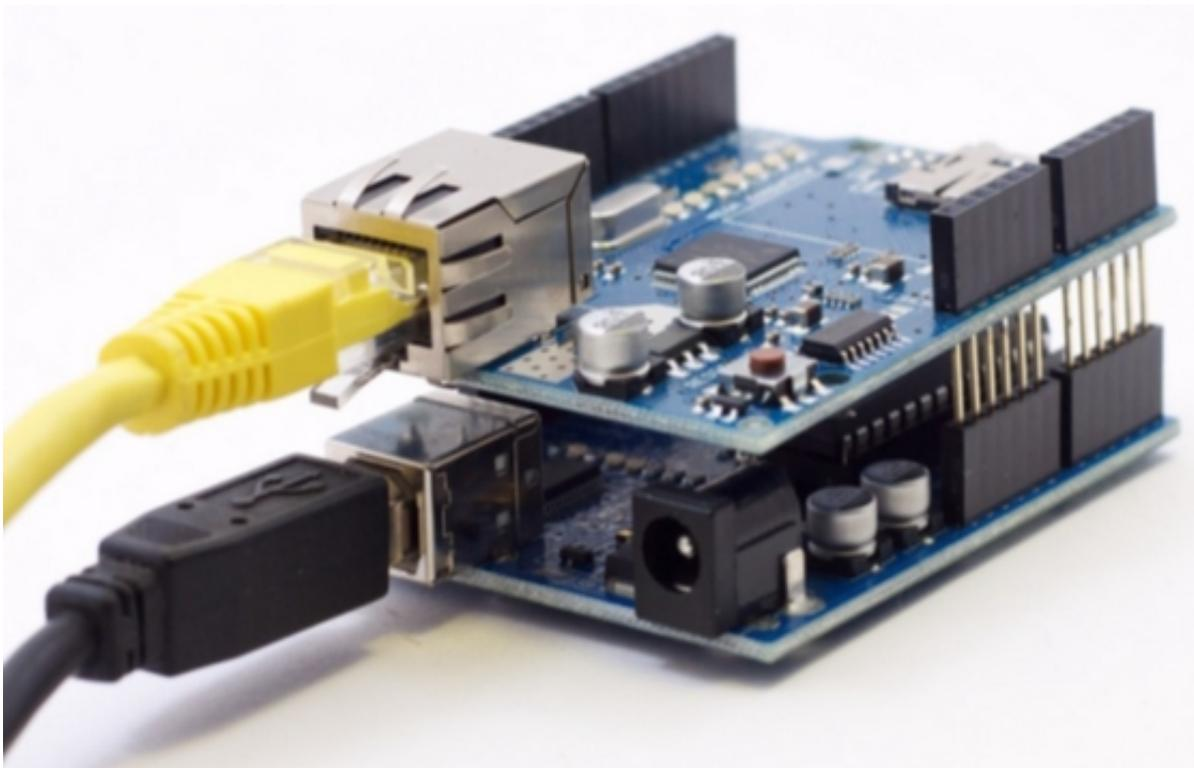
**Figure III-18.** Arduino UNO + Shield Ethernet
