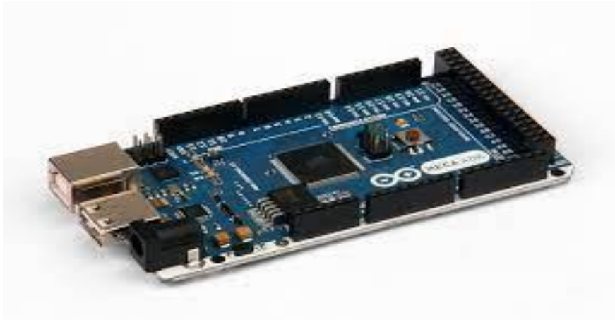
Figure II.14: La carte Arduino Mega ADK
