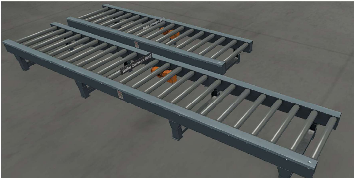
Figure III. 14: Roller Conveyor (4m, 6m).
