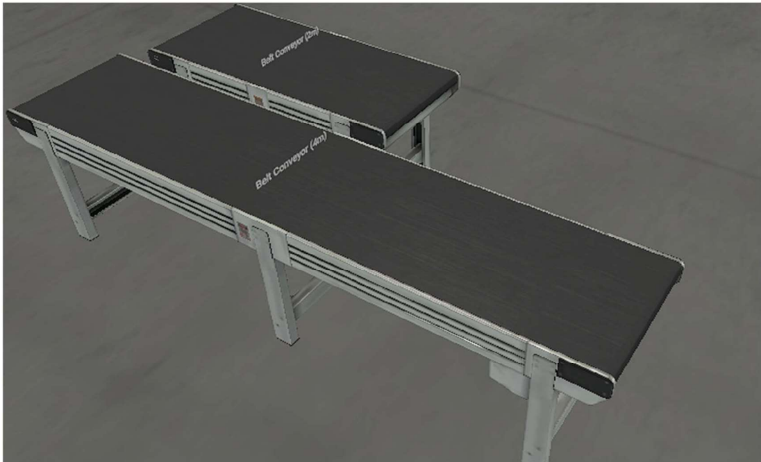
Figure III. 12: Belt conveyors (2m, 4m).
