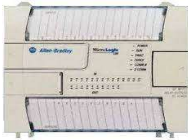
Figure I.15: Automate compact (Allen-Bradley).
