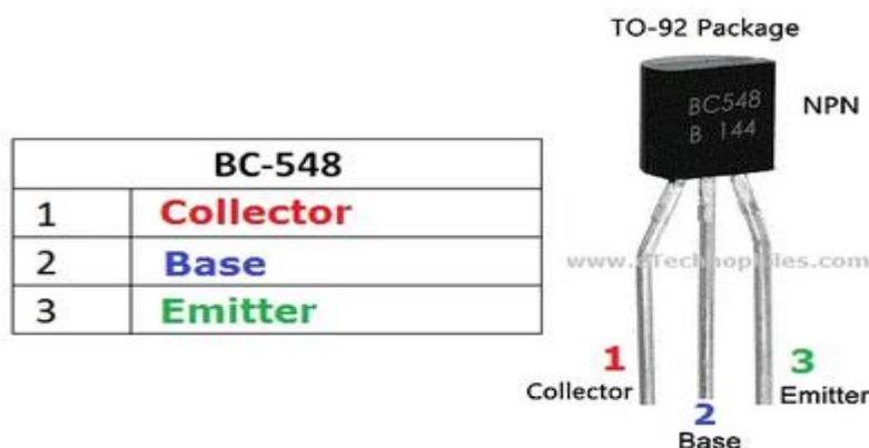
**Figure 30:** BC548 Transistor Pinout
