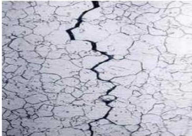
Figure 1-9 Corrosion inter granulaire
