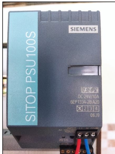
Figure 51. Alimentation SITOP PSU100S.
