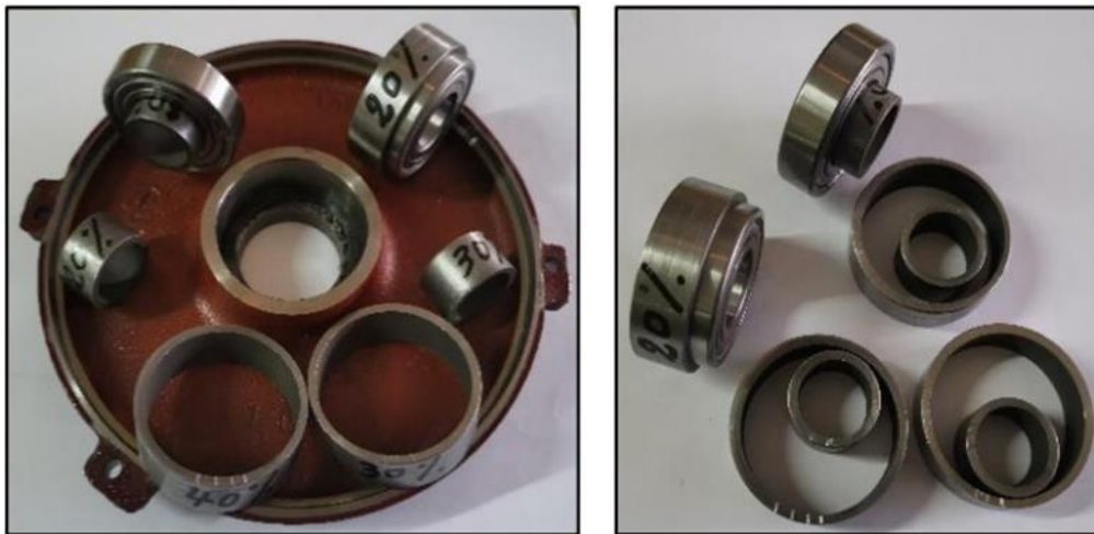
Figure IV.10. Mechanism for creating eccentricity defect
