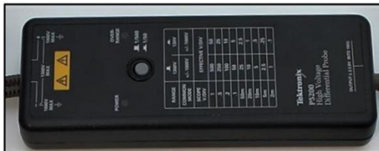
Figure IV.9. Photo of the voltage sensor used
