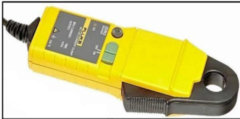
Figure IV.8. Photo of the current sensor used
