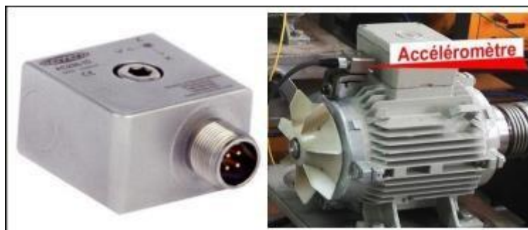
Figure I.5. Triaxial accelerometer and its location on a synchronous motor
