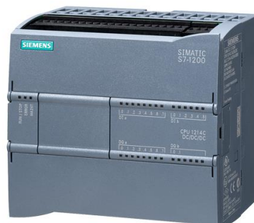
Figure III.1 : API Siemens S71200
