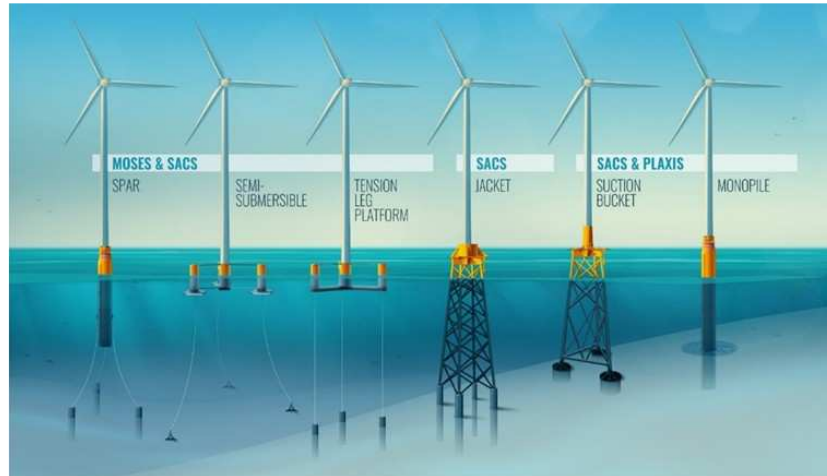
Figure I.9: Offshore wind turbines installation types. [28]
