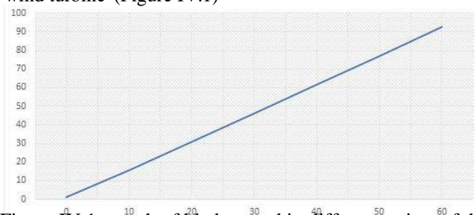
Figure IV.1: graph of blade speed in different points of the blade
