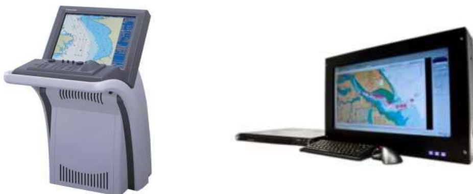
Figure III.6. Photos de la console ECDIS.
