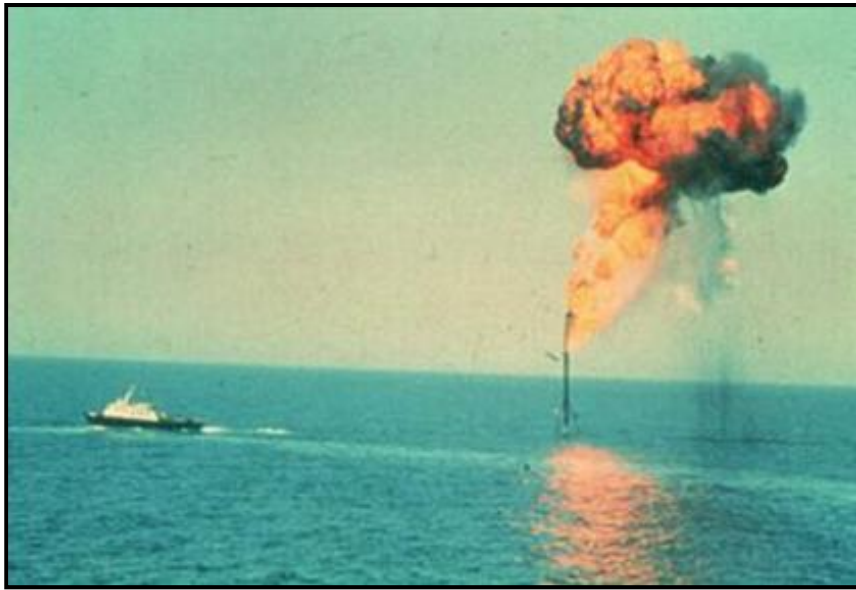
Figure 5.2.b Liquid fall out and flaming rain from flare flame.
