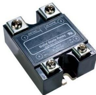
Figure II.27 Un relais statique
