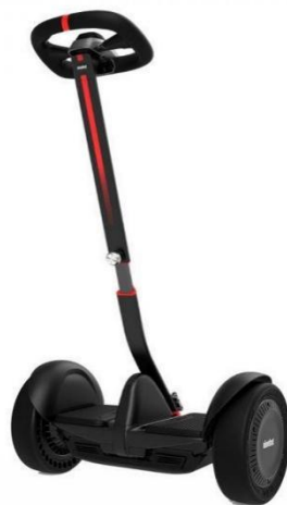
Figure I.2 : Le Segway Personal Transporter (PT)
