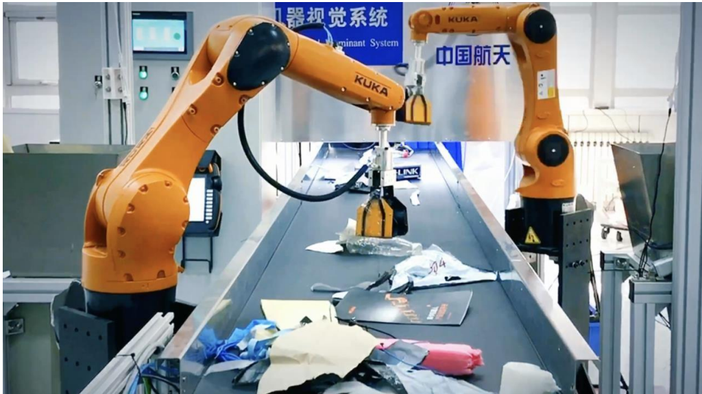
Figure 1.6. Waste sorting system
