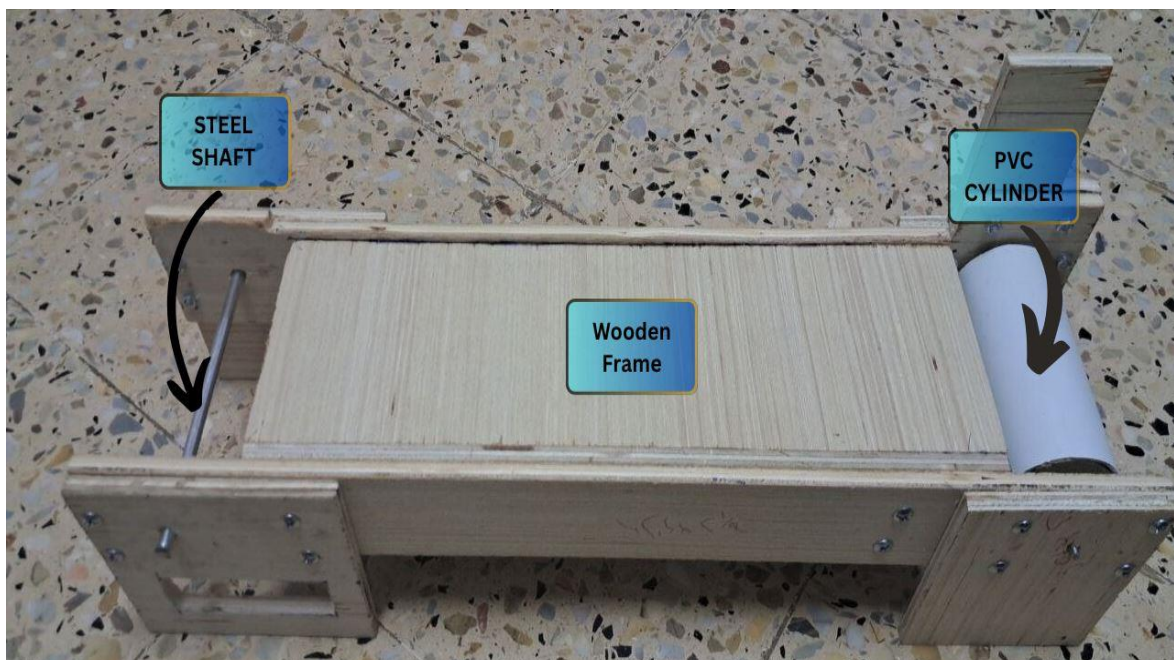
Figure 4.17. Conveyor body structure
