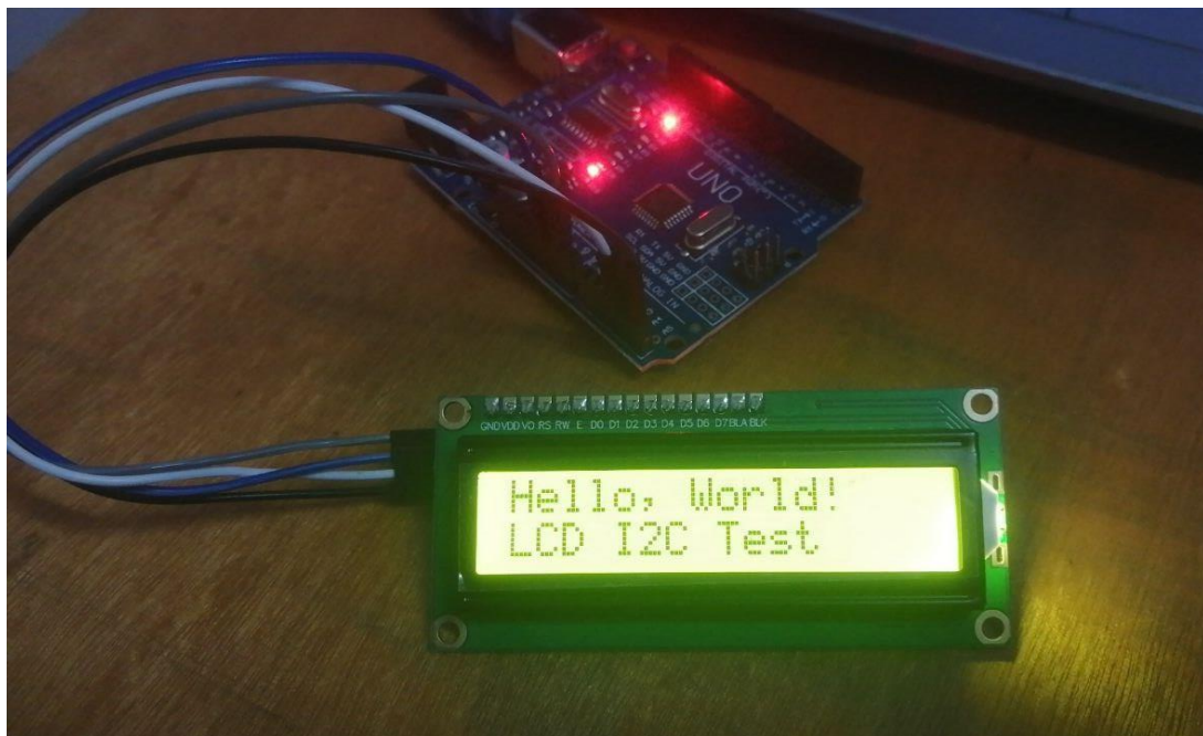
Figure 4.8. LCD I2C display test
