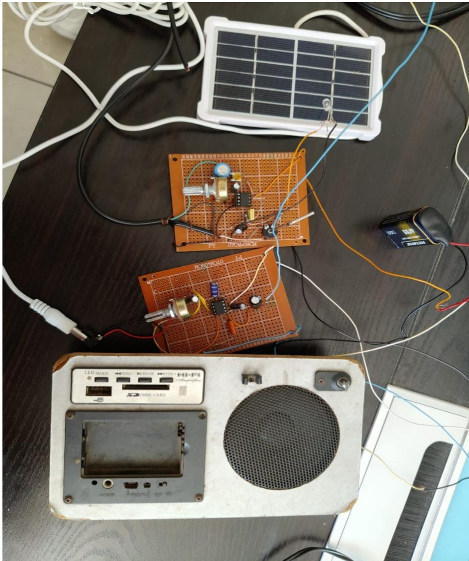
Figure 3.12: Complete Li-Fi Audio Communication System Using LM386 and Solar Panel.
