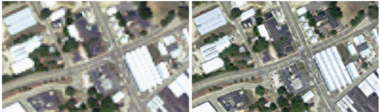
Figure 4.11. Pan-sharpening process, (left) L8 OLI_TIRS 4-3-2 color composition (30m), (right) L8 OLI_TIRS 4-3-2 color composition merged with Panchromatic 8 band (15m)
