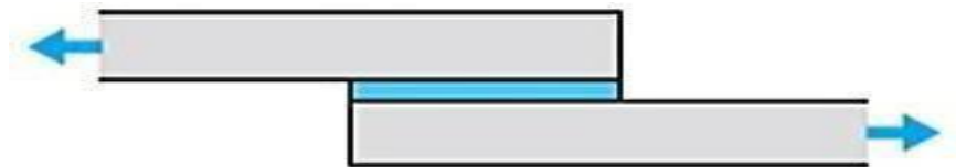
Figure 2.6: Joint à recouvrement simple
