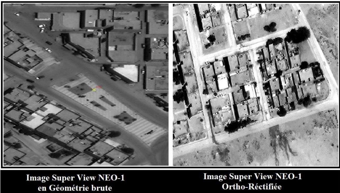
Figure 22: Illustration d'ortho rectification de l'image Super View NEO-1
